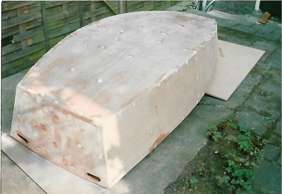
Bottom view before Epoxy and glass cloth
